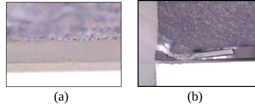
Figure 6. Failure modes after reliability tests for test vehicles mold die ; (a) de-lamination between dielectric and mold materials and (b) Mold crack
