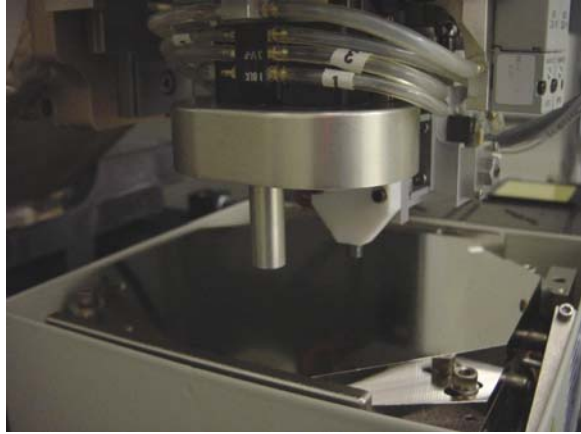
Figure 3 – Steady State Heat Wafer Stage and Pulsed Heat Pick Tool Optimized for Laser Diode Eutectic Solder Attach
