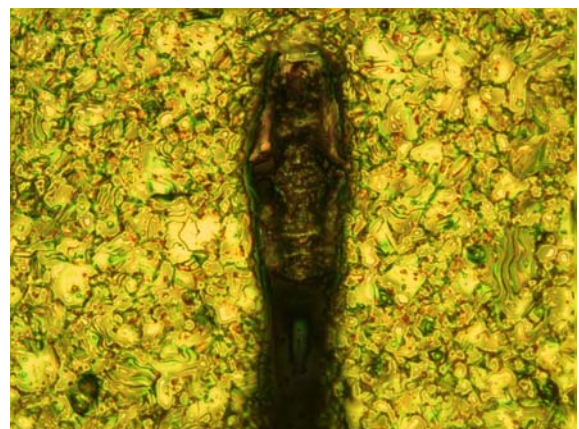
Figure 3: Wire D on LTCC (magnification 500x), tool after 26000 bonds
