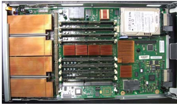
Figure 2: Inside a Blade Server; fully functional hardware with CPUs, memory, and hard drive
