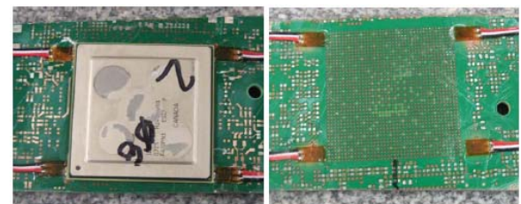
Figure 8: Uni-Axis Strain Gauge Locations
