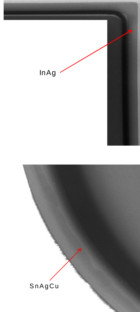
Fig. 5: Seal ring soldering in SST ovens.
