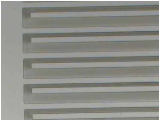
Figure 2. An Optical Photograph of the Micromachined Interdigitated Teeth Structures.
