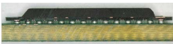
Figure 1. Single row specimen from the edge of a PBGA package. The solder balls have 1 mm pitch.
