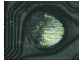
Figure 13. Ductile failure mode was observed after ball shear test in all the test conditions
