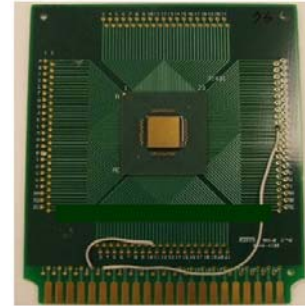
Figure 4: A typical thermal test vehicle (TTV)
