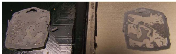
Figure 8: TTV TIM at die and heat spreader surfaces after HAST testing
