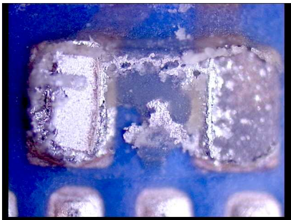
Figure 9. Chip capacitor was removed to show solder shorts beneath the capacitor.
