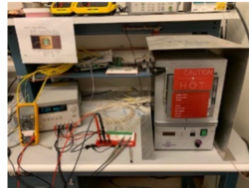
ASIC setup in 300^{\circ}\text{C} chamber, probe connections to test system (outside chamber), and test equipment
