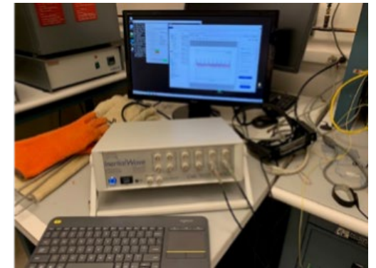
ASIC setup in 300^{\circ}\text{C} chamber, probe connections to test system (outside chamber), and test equipment
