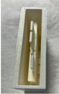
Step 1: Negative Part 3D printing
