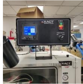
Step 3: Degassing @760mmHg In EXACT
