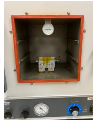
Step 8: Curing in a vacuum oven
