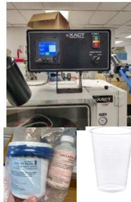
Step 7: Prepare Epoxy Resin for Degassing at 760mmHg
