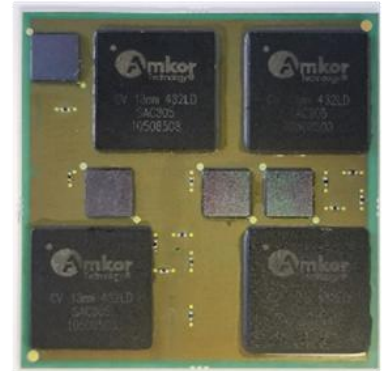
Chips Closer Together Chips Embedded in LCP
