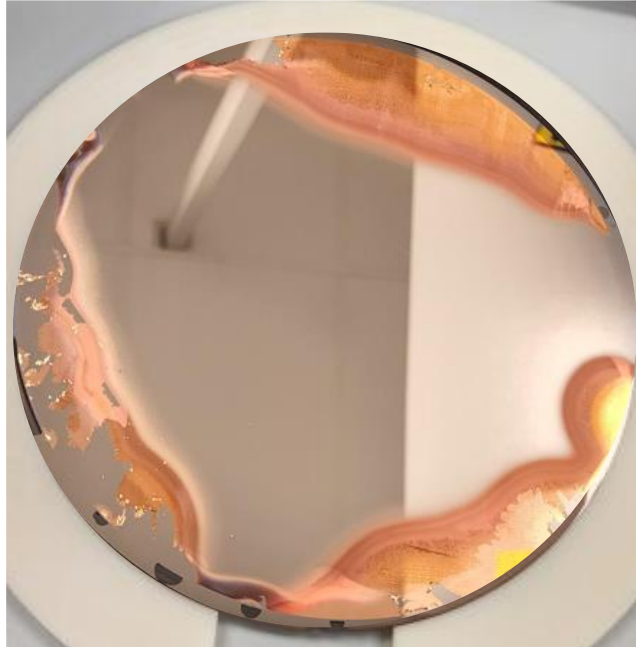
Clear delamination of Cu ECD
