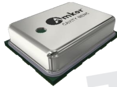
Barometer 2.5 x 2.0 mm, LGA
