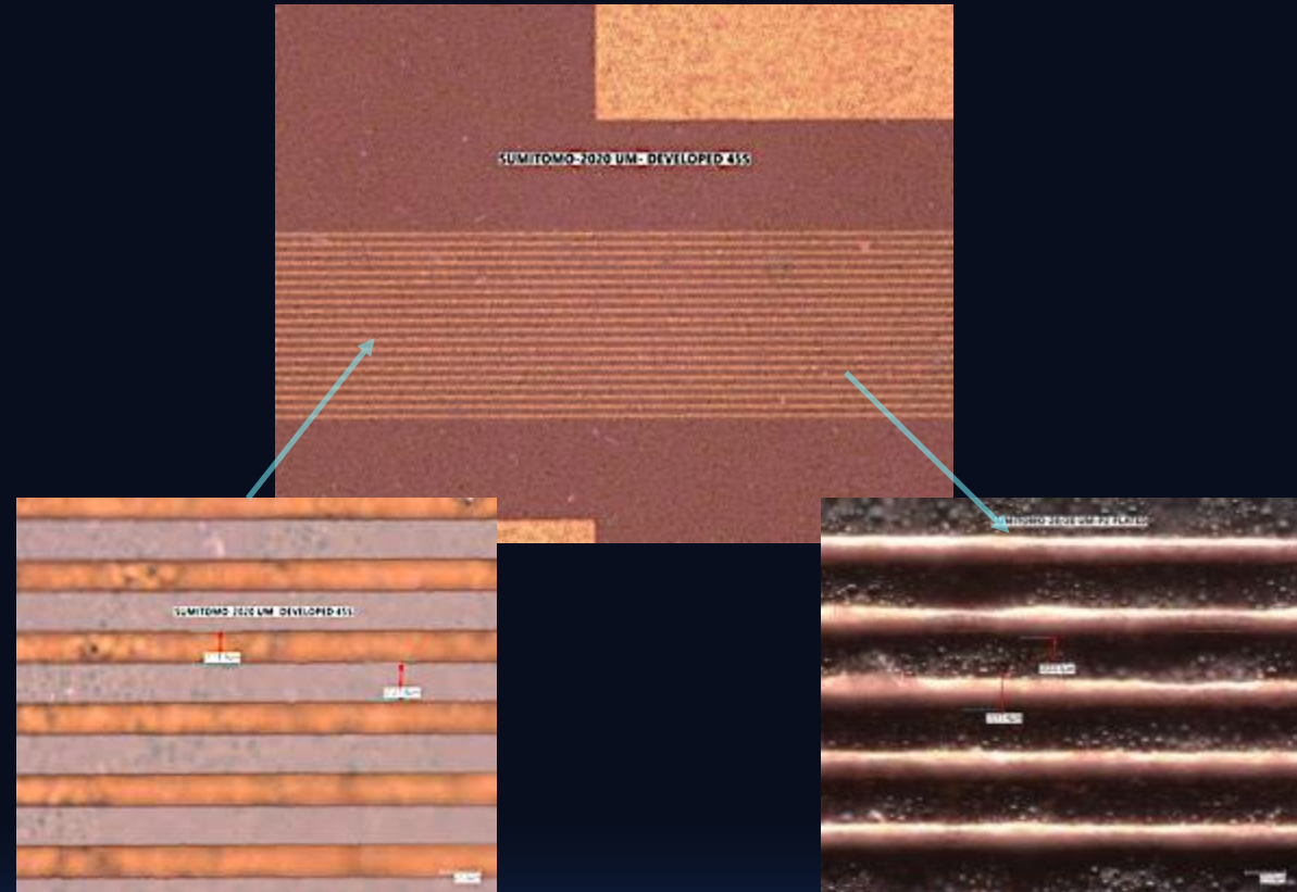
LQDX-Alconix-Brewer Science Design/Mask (7um, 15um, 20um features). Max Temp 170C.
