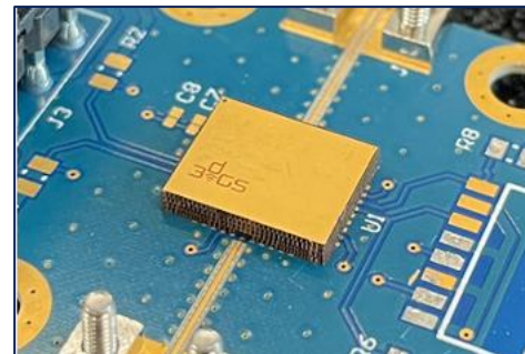
6-12GHz Half-Duplex Tx/Rx 4 3DHI Glass Layers Layer IDs: PCB, 2, 1, 2, 1
