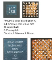
WCD9380 audio CODEC 3.0 mm x 3.1 mm x 0.47 mm 60 solder balls 0.35mm (0.40x0.40) staggered pitch Die size: 2.80 mm x 2.92 mm
