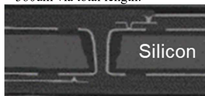
Fig. 3. Dual sided Si-Core substrate with 3 interconnect layers on top and 3 interconnect layers on bottom.
