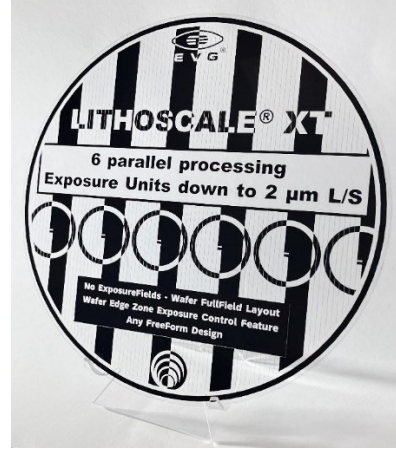
Figure 1: Glass wafer, tilted view, patterned by black resist illustrating the features of the system: six exposure heads, having fulfilled layout, wafer edge zone exposure control feature.
