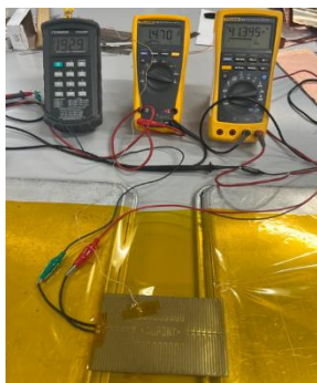
Fig. 6. (a). Pyralux® ML heater powered with attached thermocouple and multi-meter devices.
