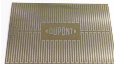
Fig. 5. Pyralux® ML heater circuit with CuNi foil
