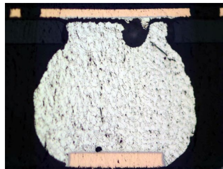
Fig. 3, Separation at device side pad has been observed.
