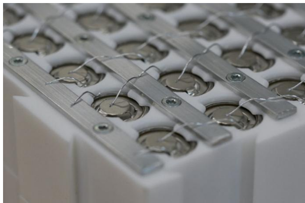
Figure 1: Aluminum wire bonded battery module.
