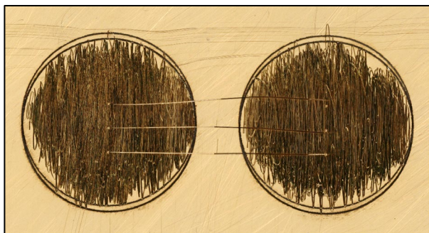
Fig. 5 - Wire Bonds and Loops Location YB, Burnished Pads
