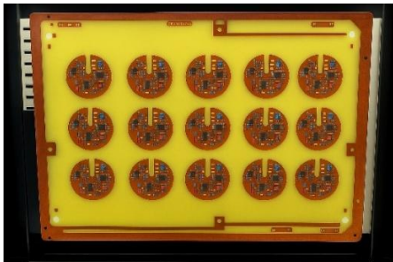
Figure 7 Inner layer of the embedded DC-DC converter module.
