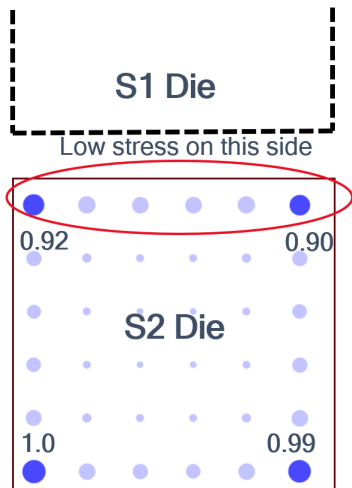
Fig. 6. Bubble plot of normalized bump stress for S2 die placed in the center with the influence of S1 die and other components. Top corner bumps showed smaller stress than bottom row due to influence of S1 die.
