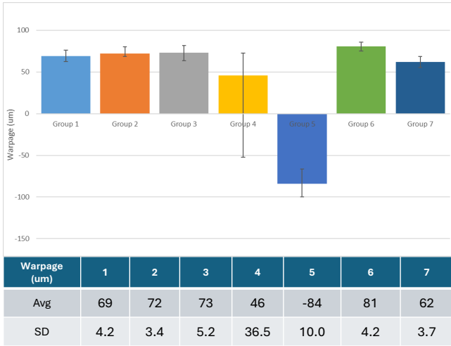
Fig. 8 Warpage results for 19 x 19 mm package at 245°C
