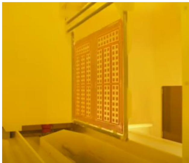
Figure 1. Glass panel Lowered into Wet Processing overflow tank in a pilot line [1]
