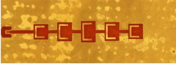
Figure 10: Fabricated 1x5 elements series-fed U-slot patch antenna test structure.
