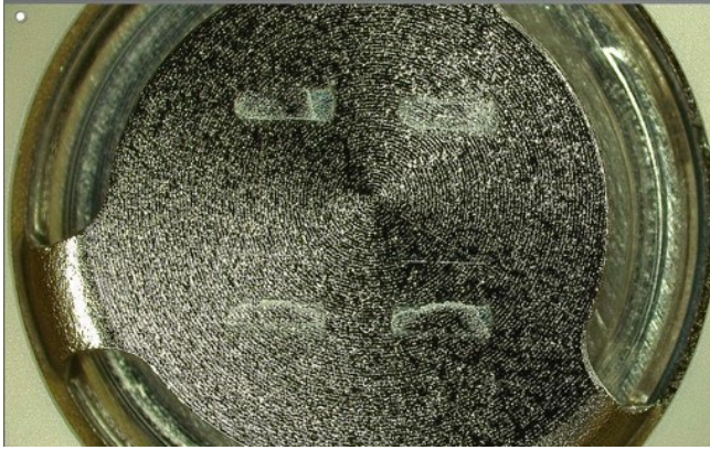
Fig. 3 Unacceptable Smart Weld Shear Nuggets
