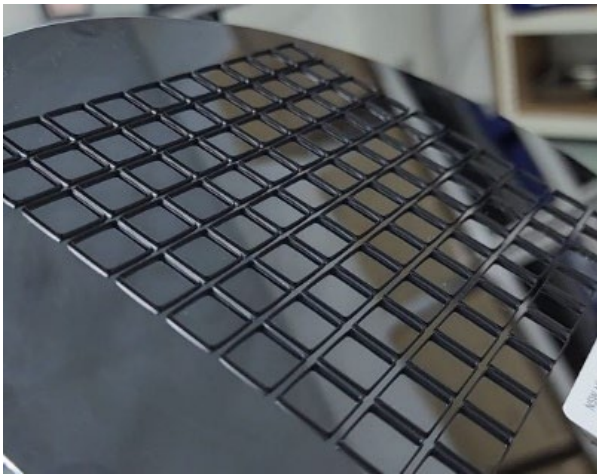
Figure 10 Investigation micro dam result on 8'' bare wafer via microscope.
