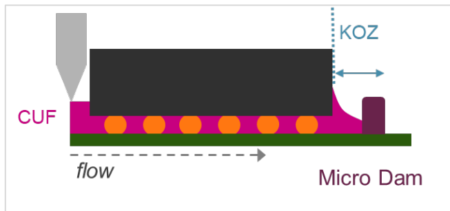
Figure 1 Schematic illustration of micro dam application as flow stop
