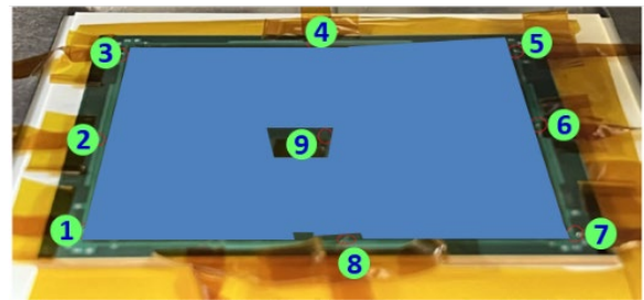
Fig. 7. Temperature monitoring positions of device-under-test by thermal couple.
