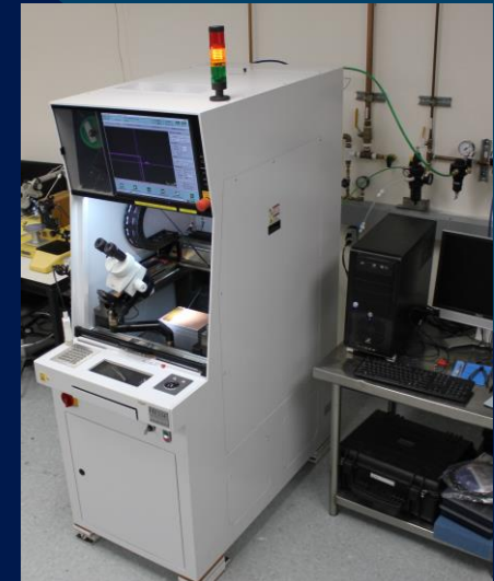
Hesse BJ935 The Bond Jet BJ935 is an ultrasonic wedge-wedge wire bonder developed for fully automated or manual processing of a wide range of substrates, chips, and other materials. Though currently configured for 12mil aluminum wire, the tool has accessories to allow for ribbon and even copper bonding..
