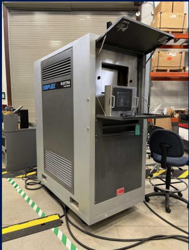
Simplex Electra 700KW Digital Load Bank This very large capacity, high performance portable load bank is designed to provide users of large AC generators and UPS systems with sophisticated testing capability. The bank features digital controllers with network control and data acquisition capability. All electrical values display on the screen and are recorded by the system for future data retrieval.
