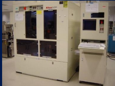
Nikon NSR2005i8A i-line stepper is a sub-micron pattern transfer tool capable of 0.5-micron resolution. Tool handling has been modified to register the pickup transparent SiC wafers during loading and unloading procedures.
