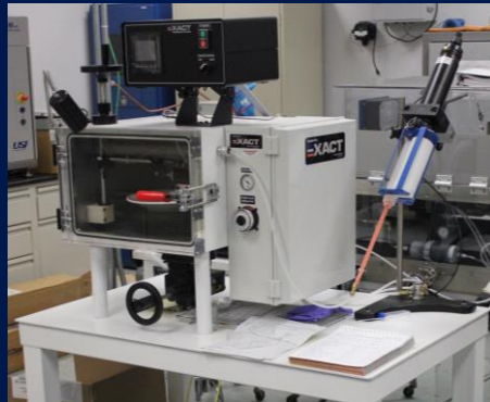
Exact Dispensing VC-18 Vacuum chamber designed to create a vacuum environment while dispensing encapsulant to insure void free coverage.
