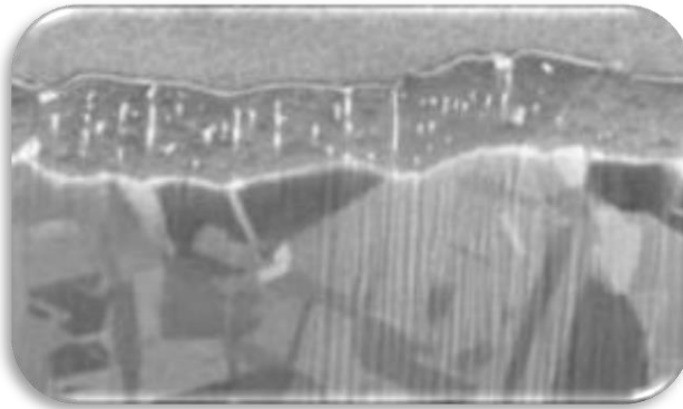
Cross section of normal tin surface as received Surface roughness S_Q > 250\text{nm}
