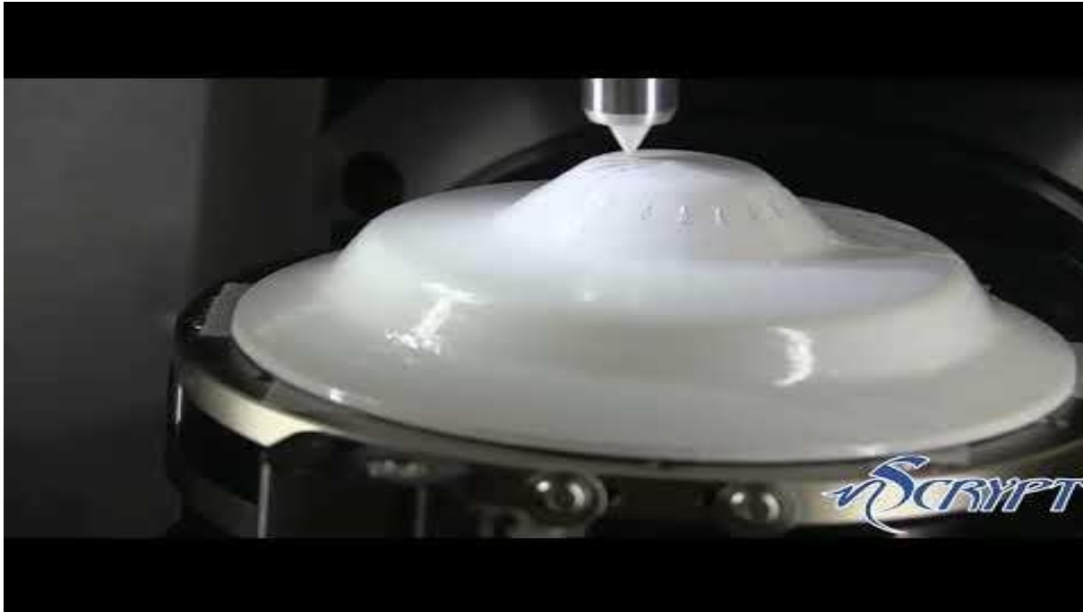
Highly Conformal Dispensing with Smartpump on Tabletop Trunnion System
