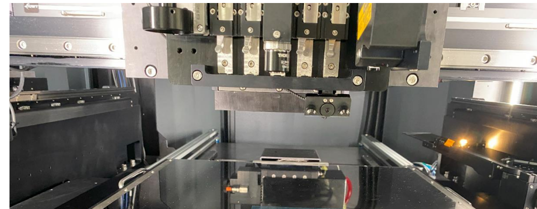
Build Plate with High Precision Axis for Movement into PulseForge Flash Area
