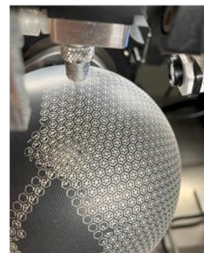
Conformal sensor circuit with Microcontroller, Bluetooth SoC, and Sensor Suite (Motion, Gas, Acoustic, etc.)
