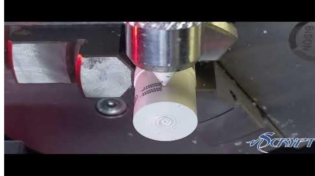
Rotary Micro-Dispensing using 4-axis Upgrade, Available on all 3Dn Systems
