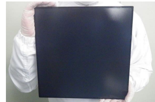
Actual panel after molding 300 mm square panel format
