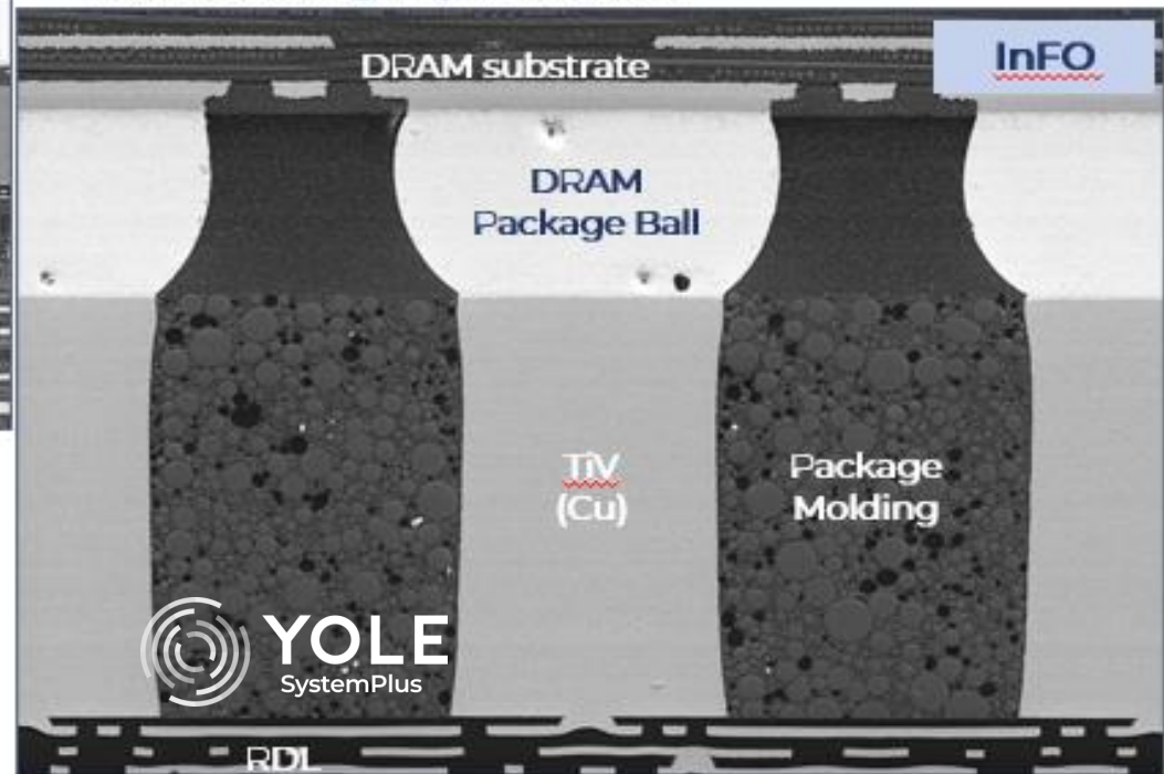
Apple A16 Package Cross-section – SEM View
