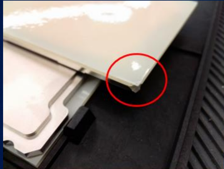
Corner chipping due to material handling
