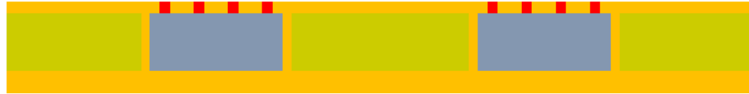
e) RDL formation by SAP Cu plating
