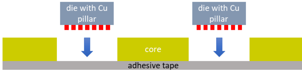
a) Placement of chips into cavities in PCB core
