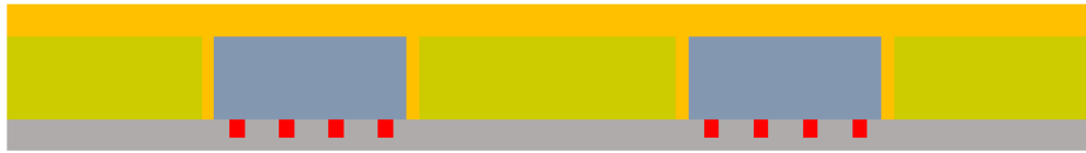
c) Removal of adhesive film & 2 nd vacuum lamination
