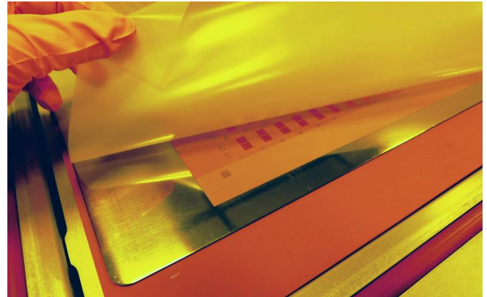
Layup for adhesive tape lamination
