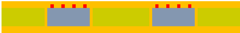
c) Removal of adhesive film & 2 nd vacuum lamination
