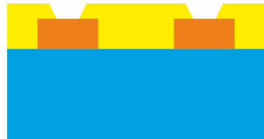
Removal of metal hard mask
