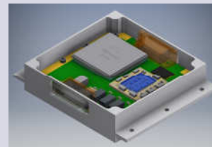
Proposed Cold Survivable Distributed Motor Controller (10cm x 10cm)
