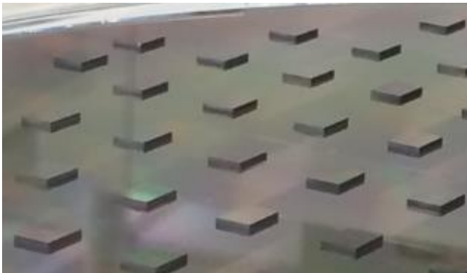
Demonstrator A - 300mm Hybrid Bonding, 5mmx7mm
