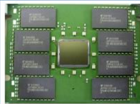
55 x 72 mm, Network Switch, ASIC + Memory
