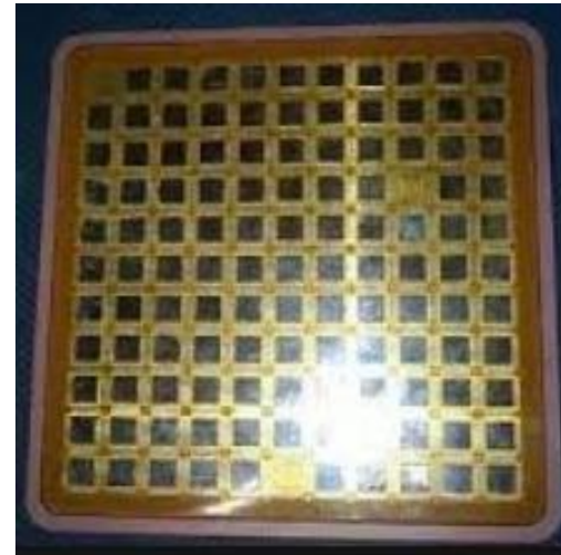
IBM 9121 TCM (Thermal Conduction Module)
