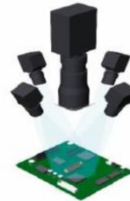
Schematic example of 3D AOI system
