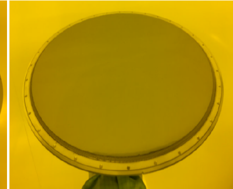
20 \mu m thinned wafer debonded
