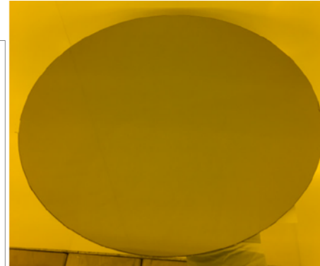
20 \mu m thinned wafer still bonded
