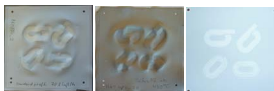
Fig. 6. Pictures of 50 µm silver coil structures in Fig. 1 in LTCC after firing unconstrained in air (left) and unconstrained under N 2 -atmosphere (center). For comparison result of a firing using constrained layer on top and bottom (right). Unconstrained sintering leads to strong warpage according to the mechanism shown in Fig. 5. In contrast to experiences with conventional Ag conductors of 10 µm thickness, firing in N 2 could not prevent the effect, presumable due to a larger amount of oxygen dissolved in the silver powder used.
