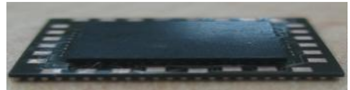
Picture of 3D eWLB PoP packages; Total less than 1.0 mm package height (including solder balls)
