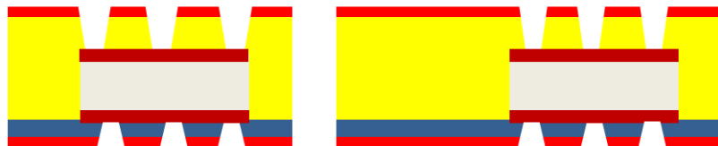
(3) Via formation to embedded die
