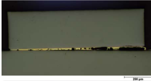
Figure 10: Optical microscopy image of a cross-section of an as bonded SLID 1b sample showing the challenges associated with co-planarity during bonding.
