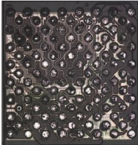
Example of Qualcomm's Audio Codec WCD9335 – eWLB package Die size: 3.6x3.6mm 2 Package size: 4.18x3.91mm 2 113 balls bumped Source: System + Consulting
