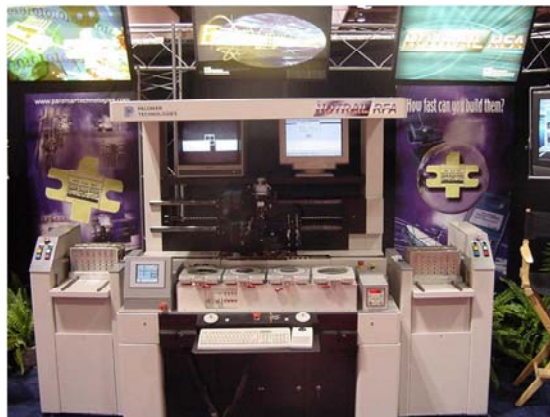
Figure 9 – Automatic Magazine to Magazine Header Load/Unload and 4 Wafer Frame/Grip Ring RFSOE Eutectic Assembly Cell
